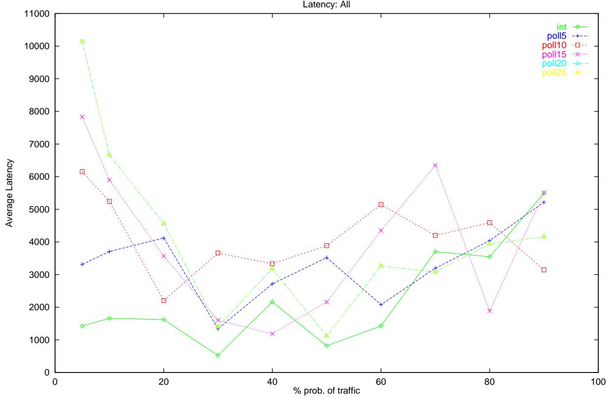
This graph illustrates several important points. First, for large inter-arrival times (low 200us probability of sending — the left side of the graph), interrupt mode has, on average, lower latency than the polling modes. This happens because, in interrupt mode, immediately after a packet arrives, the CPU is interrupted. In polling mode, the NIC must wait to be polled at the next interval; this increases the average latency.
