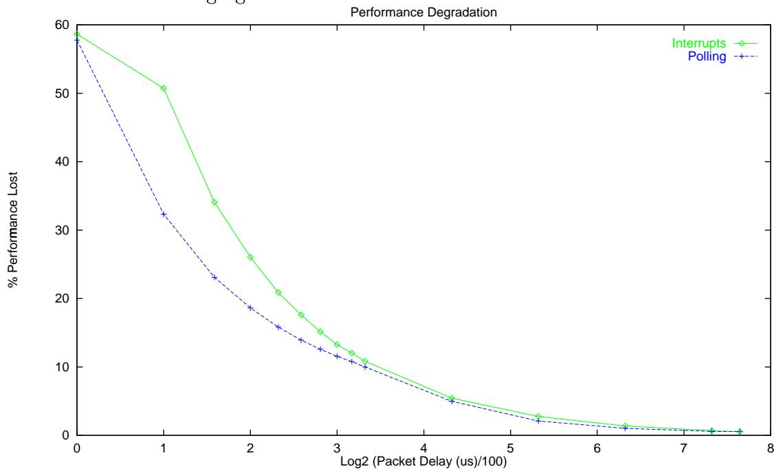
The graph above shows the CPU overhead as a function of inter-arrival time compared to a baseline (100%) with no network traffic. To better illustrate the difference, the X-axis is log-based: the first data-point (0) corresponds to 100us, 1 to 200us, 2 to 400us, ..., and 8 to 25.6ms.
